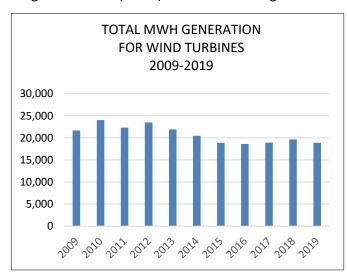
lower level of about 19,000 MWh. The turbines were commissioned in the spring of 2004 and are approaching 16 years of operation. They produce between 7% and 8% of ARPA's energy needs.
